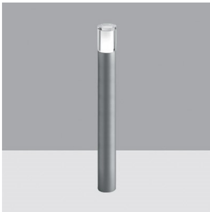
EX8 MANUFACTURER: IGUZZINI LANTERN: IPOINT COLOUR TEMPERATURE: 2900K OPTIC: DIFFUSED LIGHT POWER: 14.4W LED PER M FIXING: 1M ROOT MOUNTED TILT APPLIED: 0° MAINTENANCE FACTOR: 1 ELECTRONIC CONTROL GEAR
