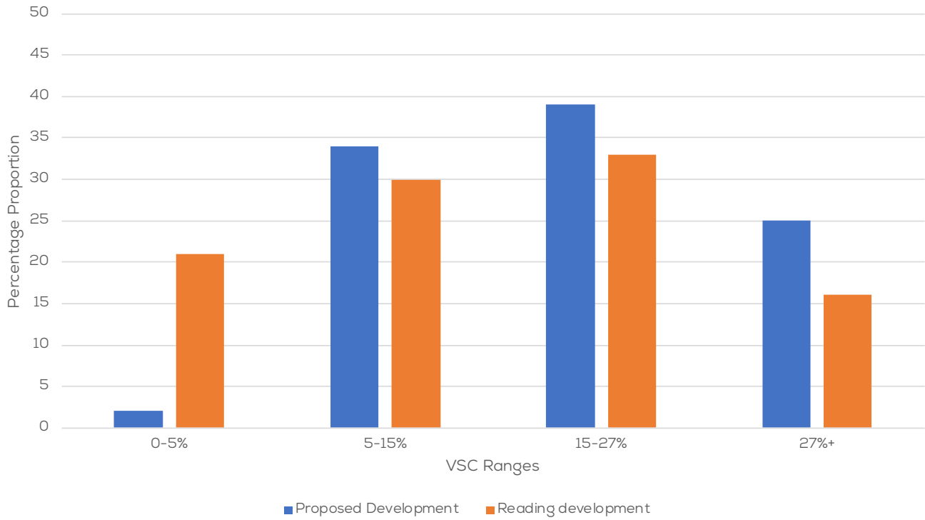
Fig. 30: Comparative analysis of retained VSC values from the Proposed Development with retained VSC values in the Reading Study Area
