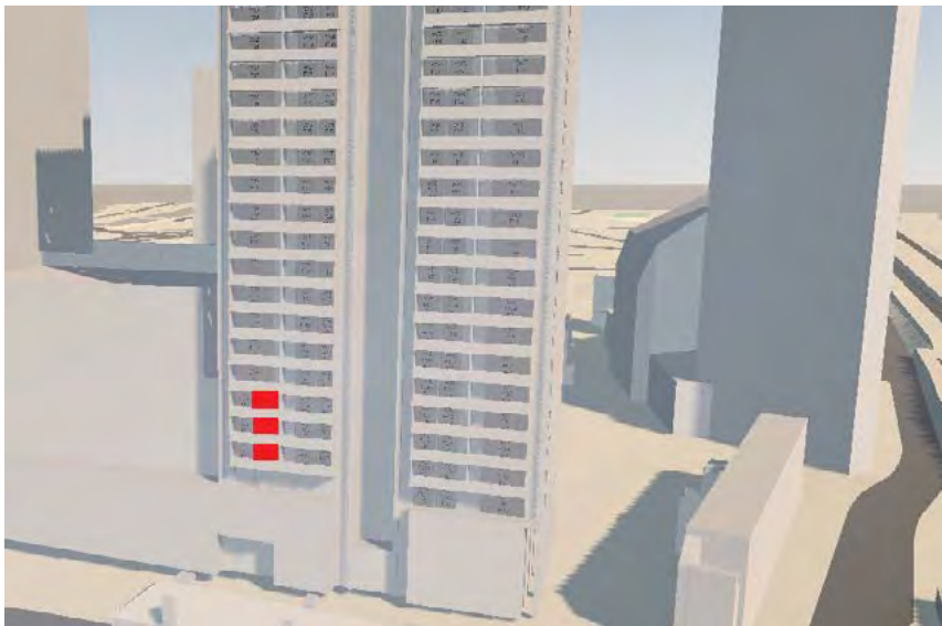
Fig. 148: Window map showing three windows which fall short of their winter sunlight target in the “no-balcony” scenario
