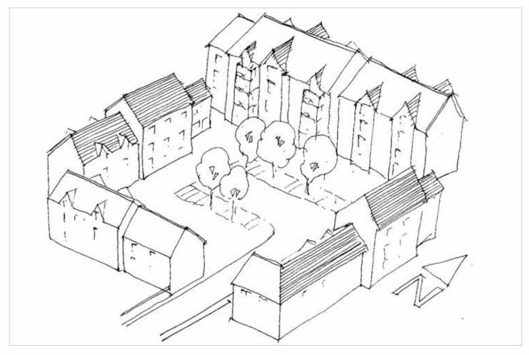
Fig.28 Place taller buildings towards the northern section of the site and lower buildings towards the south to make the most of passive solar gain and avoid overshadowing.
