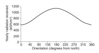
Figure 37: Solar radiation received on a  $45^{\circ}$  slope, for London
