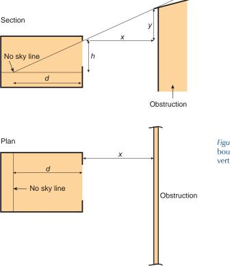
*Figure D3:* For a long horizontal obstruction parallel to the window, the no sky line is also parallel to the window. Its position can be found from the section.
