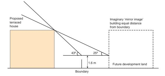
Figure 22: Derivation of an angular boundary criterion to safeguard future development of adjoining land
