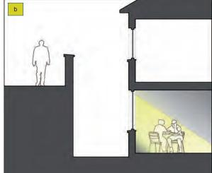
*Figure 4:* Daylight penetration in a basement (a) is improved by a raised window head (b)
