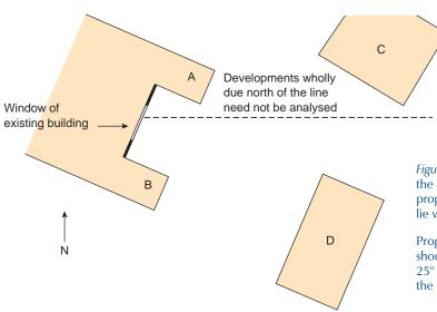
*Figure 27:* In analysing the sunlighting impact on the existing window, no check need be made for proposed extension A and new building C, as they lie within 90° of due north of the window.
