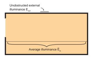
*Figure 5*: Definition of ADF. Under standard overcast conditions:
