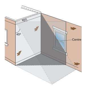
*Figure 17:* Application of the 45° approach to a domestic extension. A significant amount of light is likely to be blocked if the centre of the window lies within the 45° angle on both plan and elevation. Here the centre of the window lies outside the 45° angle on elevation, so the impact of the extension is likely to be small.
