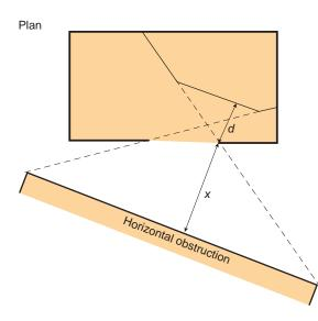
*Figure D6:* For a general horizontal obstruction, part of the no sky line runs parallel to the obstruction. The rest runs along the projected lines from the ends of the obstruction through the corners of the window.
