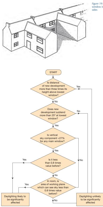
*Figure 19:* A tunnel effect can occur if a window is obstructed by extensions on both sides
