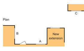
*Figure 16:* To assess the impact of the new extension, the  $45^{\circ}$  approach may be used for window A but not for windows B and C which directly face it
