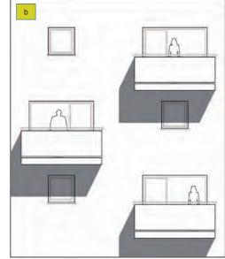
*Figure 12:* In a conventional layout (a) the balcony above each living room reduces the daylight it receives. Staggered balconies (elevation b) give improved daylight and sunlight to living rooms.
