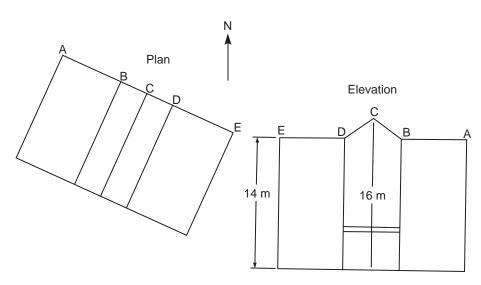
Figure G4: Outline plan and elevation of a shadow plotting example building
