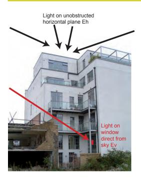
*Figure 2:* The vertical sky component is the illuminance on the outside of the window, divided by the illuminance on an unobstructed roof, under overcast sky conditions. Reflected light is not included.
