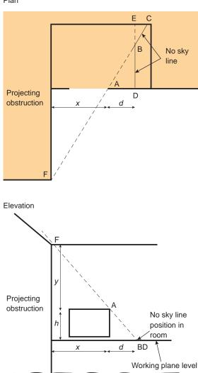
*Figure D5:* For a horizontal obstruction projecting from the window wall, the no sky line runs partly parallel to the obstruction and partly along a continuation of the line joining the end of the obstruction F and the side of the window A
