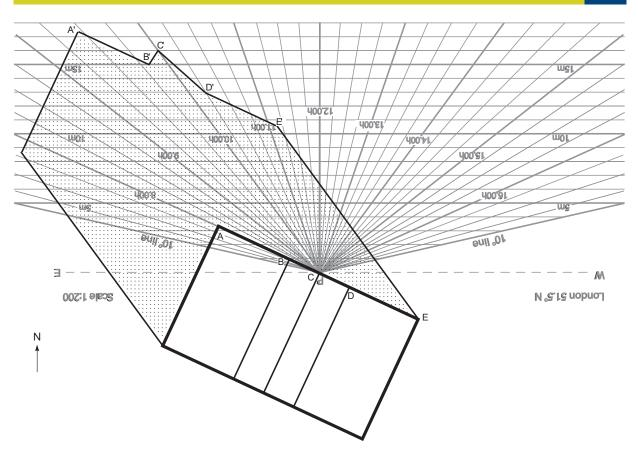
Figure G5: Use of the sun-on-ground indicator to plot the shadow of the example bulding in Figure G4 on 21 March
