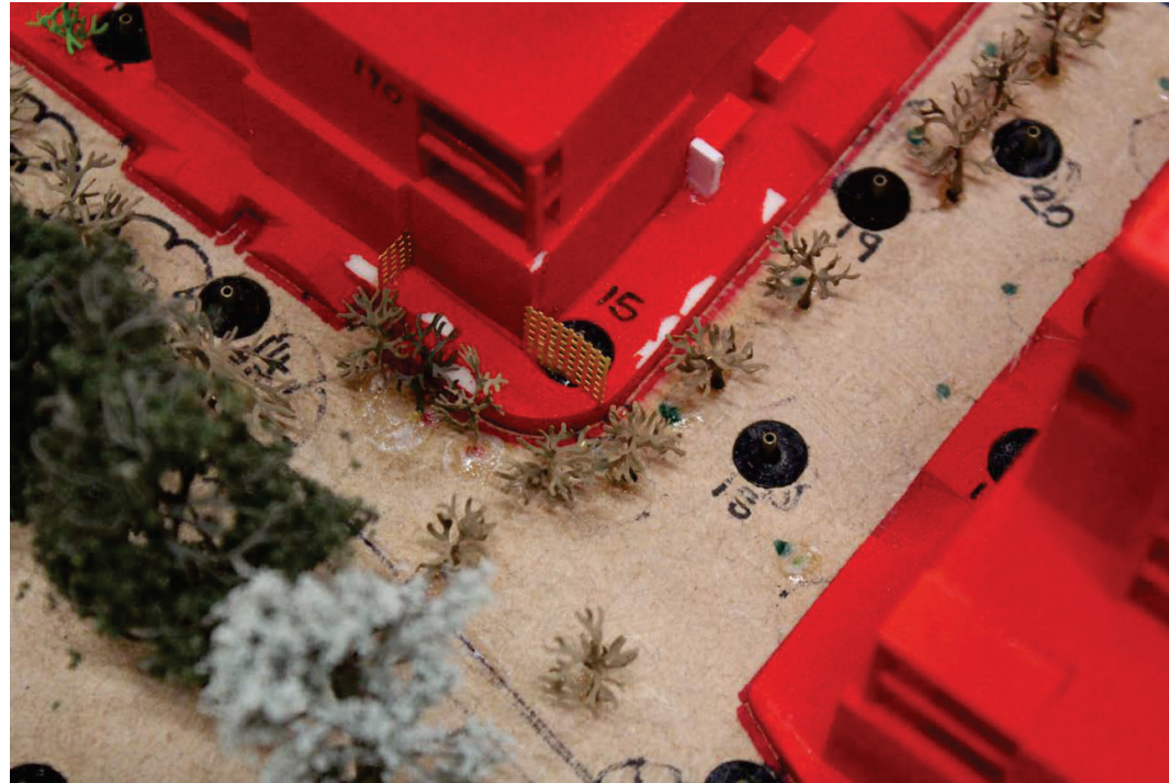
Figure 38: Image showing three, 5m tall, deciduous trees at the south-east corner of Block 4, a 3m tall 50% porous screen separating entrances at the south façade of Block 4, and a 3m tall, 5m wide 50% porous screen extending eastward from the eastern façade at the south-east of Block 4
