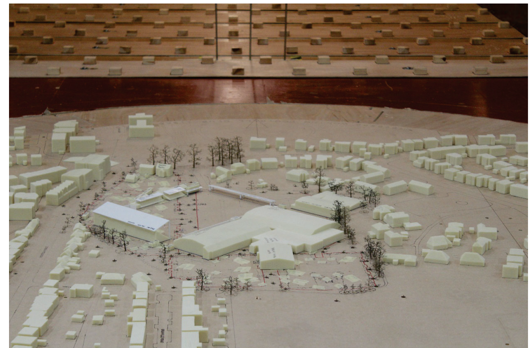
Figure 25: Existing Site and Surrounding Buildings (Configuration 1) - View in the Wind Tunnel (from the South)
