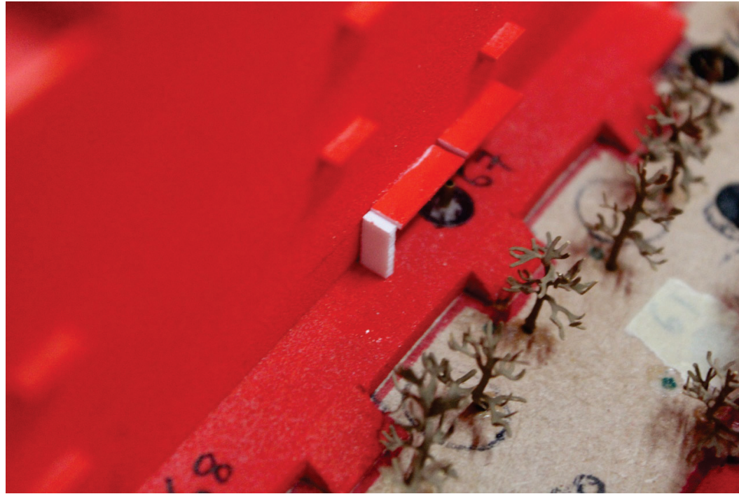
Figure 34: Image of 3m tall, 1.5m wide, solid side screen added to canopy above entrance location at southern façade of Block 2
