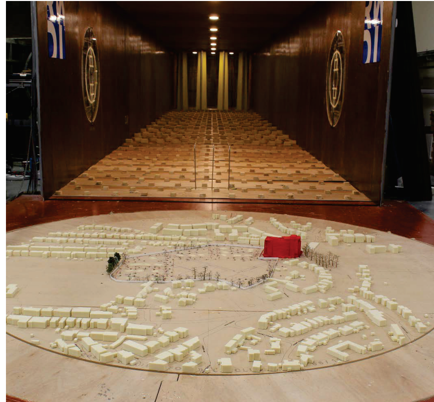
Figure 26: Proposed Development and Existing Surrounding Buildings (Configuration 2) - View in the Wind Tunnel (from the East)
