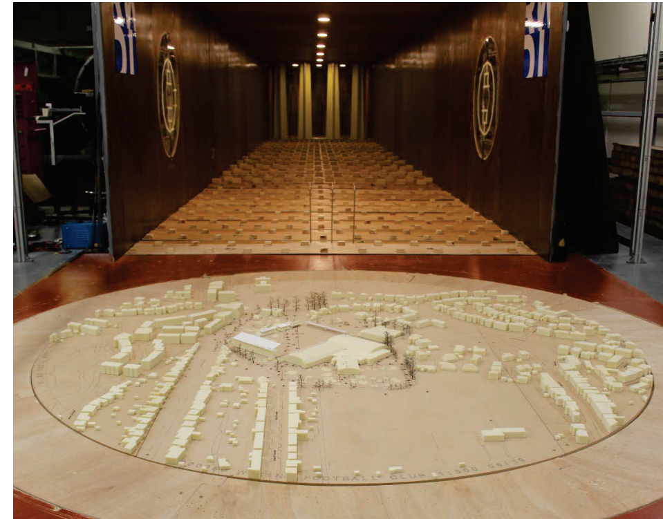
Figure 24: Existing Site and Surrounding Buildings (Configuration 1) - View in the Wind Tunnel (from the South)
