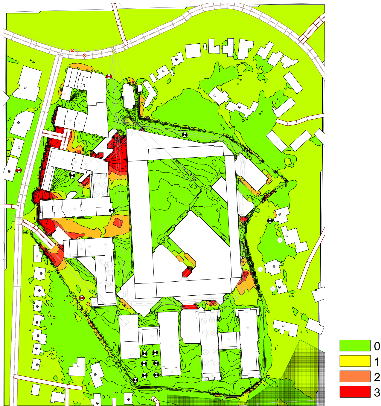
Figure 9.13 Comparison of 2025 Future Road with the Proposed Development and Without the Proposed Development (light green = no increase in noise level dB, white = buildings demolished, existing or proposed)
