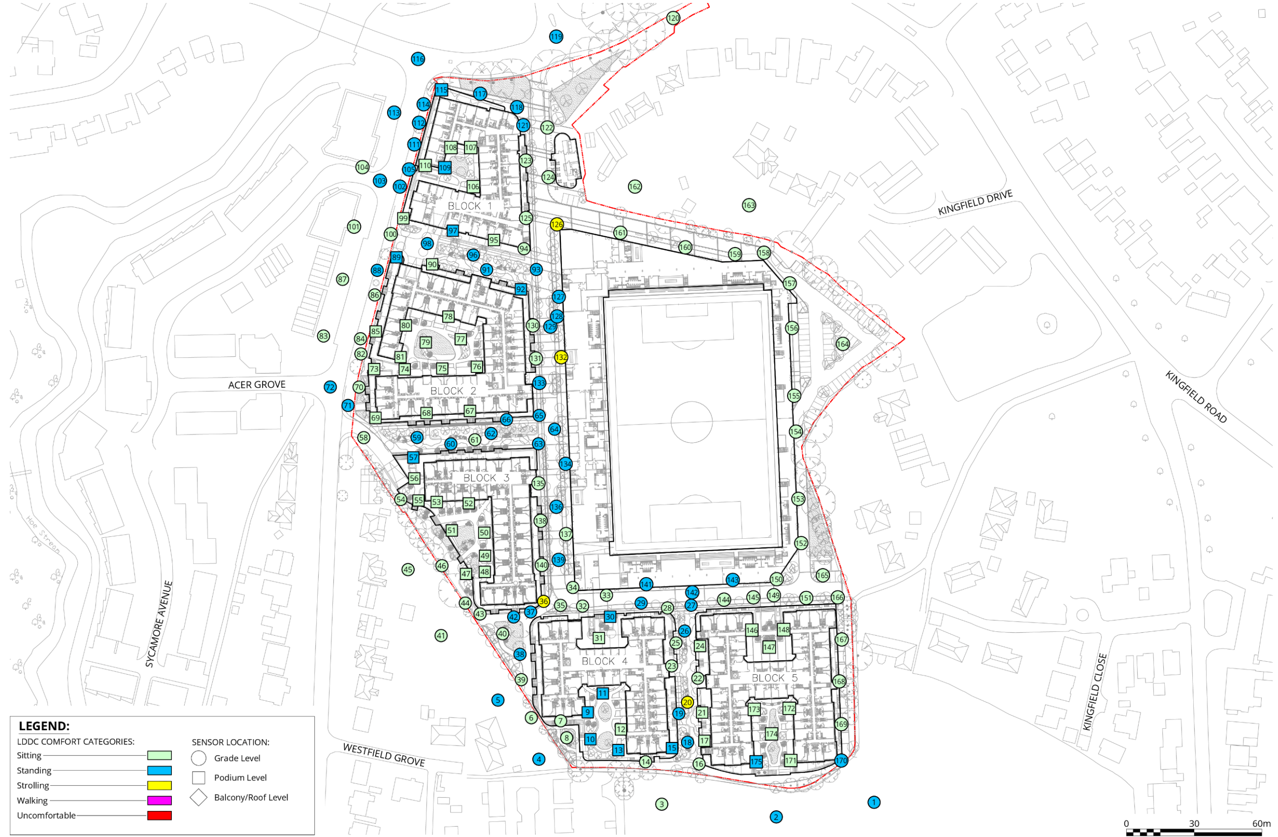
Pedestrian Wind Comfort Conditions - Ground Floor and Podium Level Configuration 4: Proposed Development with Existing Surrounding Buildings and Proposed Landscaping Scheme and Mitigation Measures Summer Season
