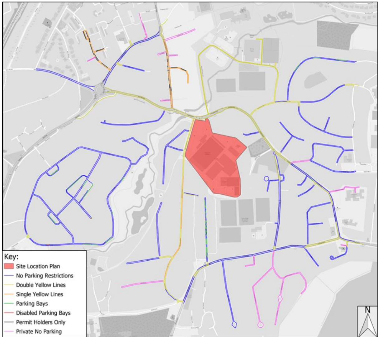
Figure IS5 – Existing Car Parking Restrictions on Streets Around the Stadium
