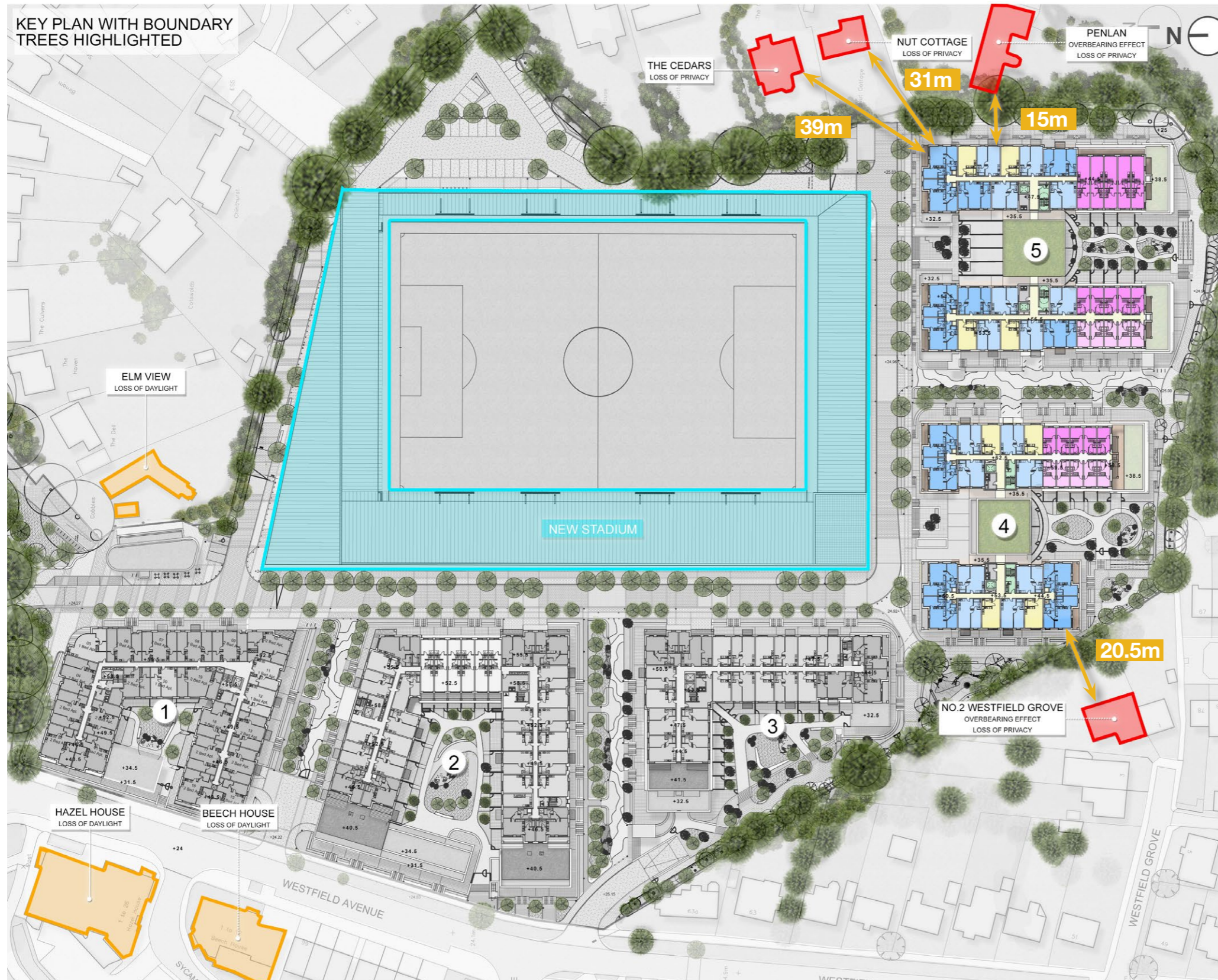
FIGURE 3 : Diagram illustrating the identified properties and the closest separation distance to a window on the Proposal
