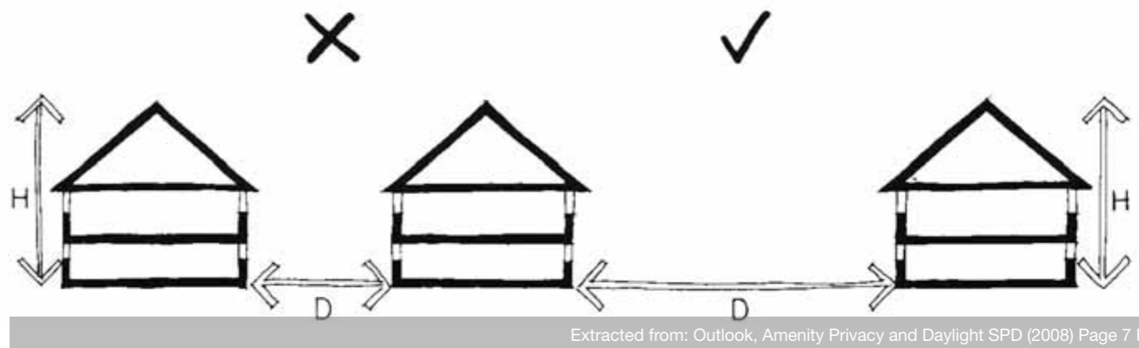
FIGURE 143: Diagram illustrating examples of outlooks and separation distances from SPD
