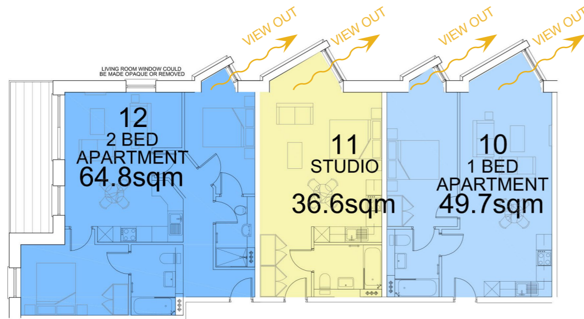
FIGURE 128: Plan Showing possible angled Window Solution On Block 5 Elevation
